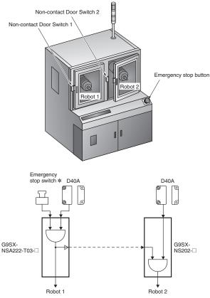
\* A manual reset is required when an emergency stop is used.
