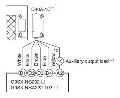
\*1. The auxiliary output load current must be 10 mA max.
