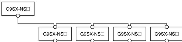
2. Any G9SX-NS□ Controller that receives a logical AND connection input can be logically connected to other Controllers on up to five layers.
