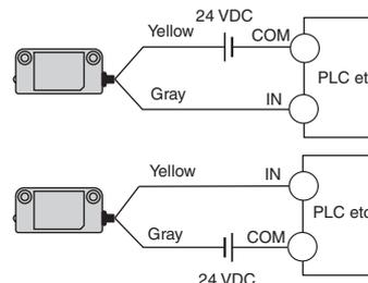
**Note:** The auxiliary output load current must be 10 mA max. Wrong connection may lead to a failure of the auxiliary output circuit.
