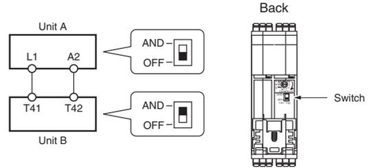
**Note:** A setting error will occur and Unit B will lock out if the logical AND setting switch on the Unit B is set to OFF.
