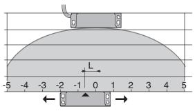
5 mm misalignment tolerance after setting
