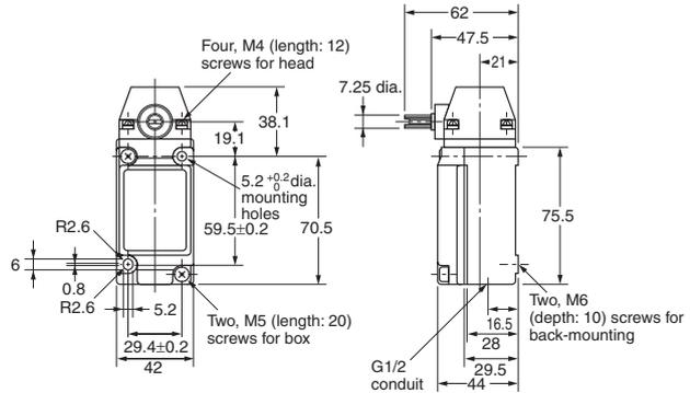
Note: Unless otherwise specified, a tolerance of  $\pm 0.4$  mm applies to all dimensions.
