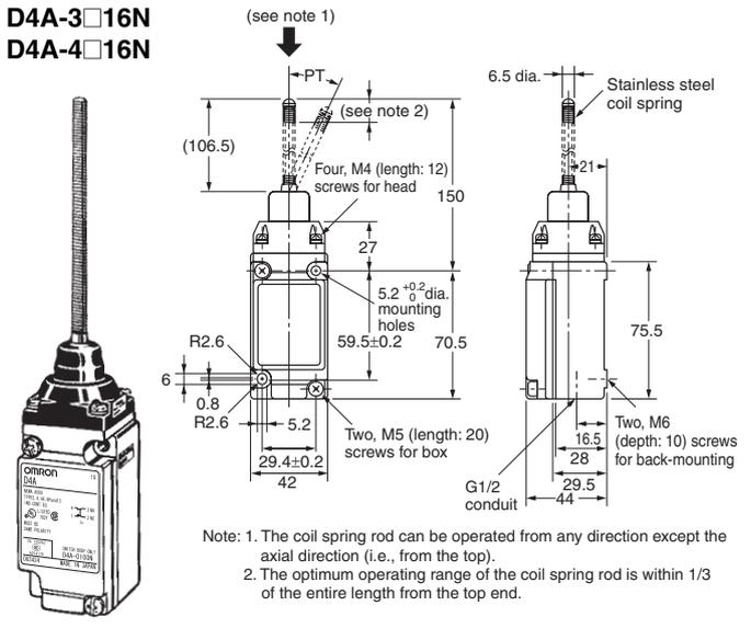
Note: Unless otherwise specified, a tolerance of ±0.4 mm applies to all dimensions.
