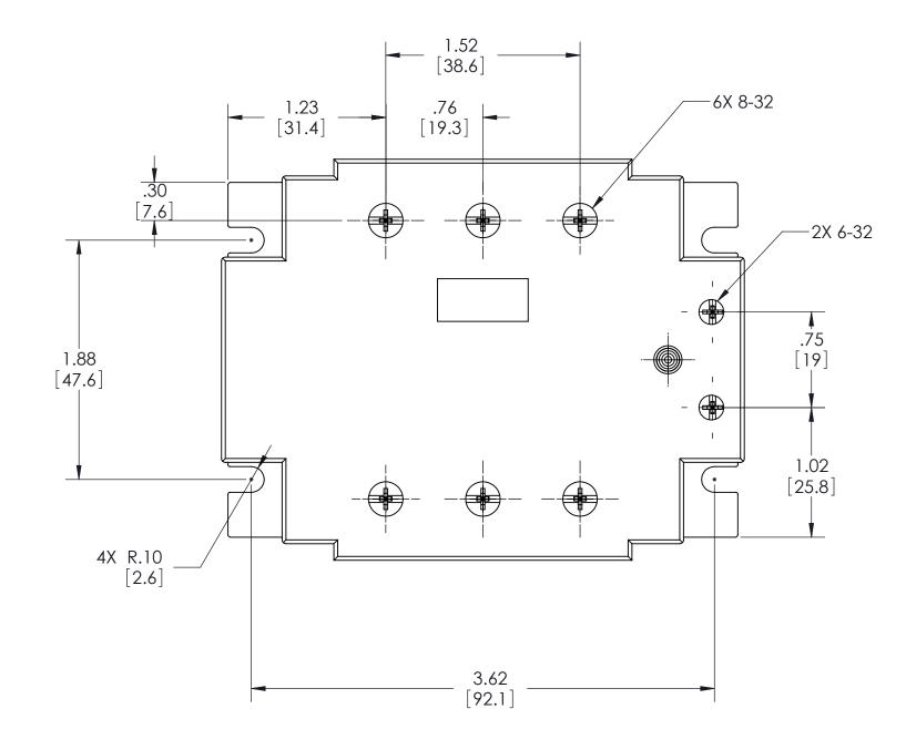
Tolerances: ± 0.02 in / 0.5 mm. All dimensions are in: inches [millimeters]
