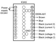
Note: Two inputs are possible on the K3AS, however, due to the output circuit of the D5SN, two current inputs are not possible.
