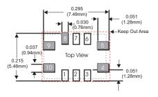
\* Do not route any traces in the keep out area. It is recommended the next layer under the keep out area is to be ground plane.
