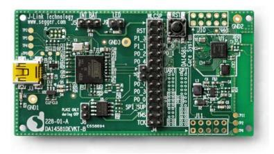
This Basic development kit gives you all flexibility to develop with confidence. All of the DA14581's I/Os are available and mapped on to expansion connectors. A debugger is provided on the PCB which in combination with SmartSnippets<sup>™</sup>, Dialog's complete software environment, enables you to program and test your A4WP or HCI application.
