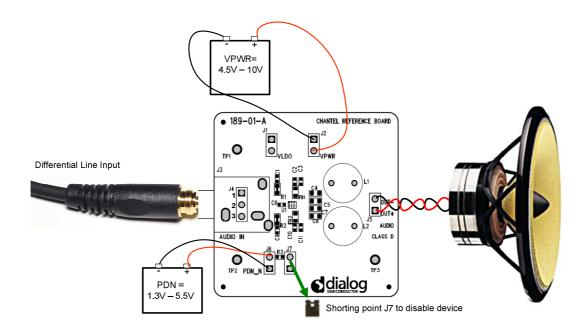
Figure 2: DA7202 performance EVB external connections
