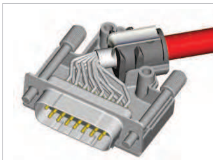
Mount connector and cable into the backshell
