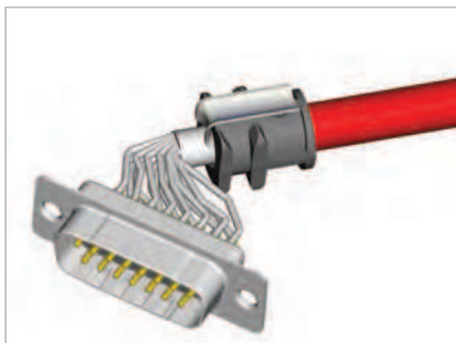
Bend cable shielding back on outside of strain relief
