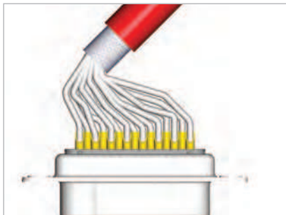
Strip cable 18mm and shape cable to two pigtails
