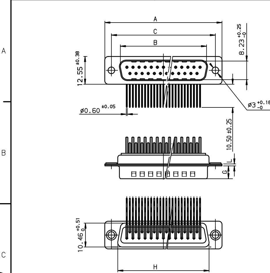
Dimensions are in millimeters
