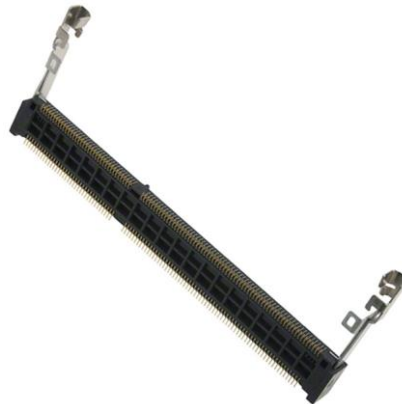
Fig. 6 A photo of the standard 204 pin DDR3 SODIMM connector
