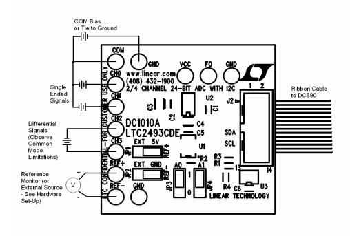
Figure 1. Proper Measurement Equipment Setup
