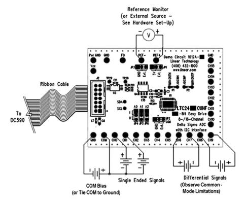
Figure 1. Proper Measurement Equipment Setup
