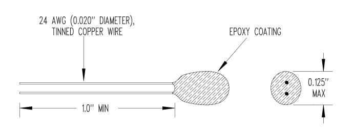
RESISTANCE @  $+25^{\circ}C = 10,000 \Omega \pm 2\%$ RESISTANCE/TEMPERATURE CURVE = "G" BETA " $\beta$ " (0 TO  $+50^{\circ}C$ ) = 3,575 K NOMINAL TEMPERATURE COEFFICENT @  $+25^{\circ}C = -4.04\%$  C NOMINAL DISSIPATION CONSTANT = 3 mW/°C NOMINAL THERMAL TIME CONSTANT = 15 SECONDS MAXIMUM (STILL AIR) THERMAL TIME CONSTANT = 3 SECONDS MAXIMUM (STIRRED OIL) MAXIMUM TEMPERATURE RATING =  $+150^{\circ}C$
