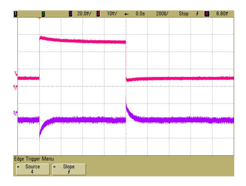
Figure 3. Load Step Response  $V_{_{IN}} = 2.5 V, \ V_{_{BIAS}} = 5 V \ V_{_{OUT}} = 1.5 V, \ 400 \ mA \ Load \ Step \ (100 \ mA <-> 500 \ mA)$
