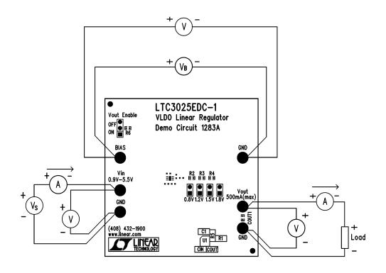
Figure 2. Proper Measurement Equipment Setup
