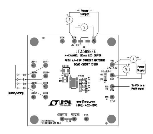
Figure 1. Proper Measurement Equipment Setup
