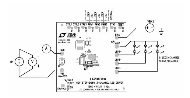
Figure 1. Proper Measurement Equipment Setup
