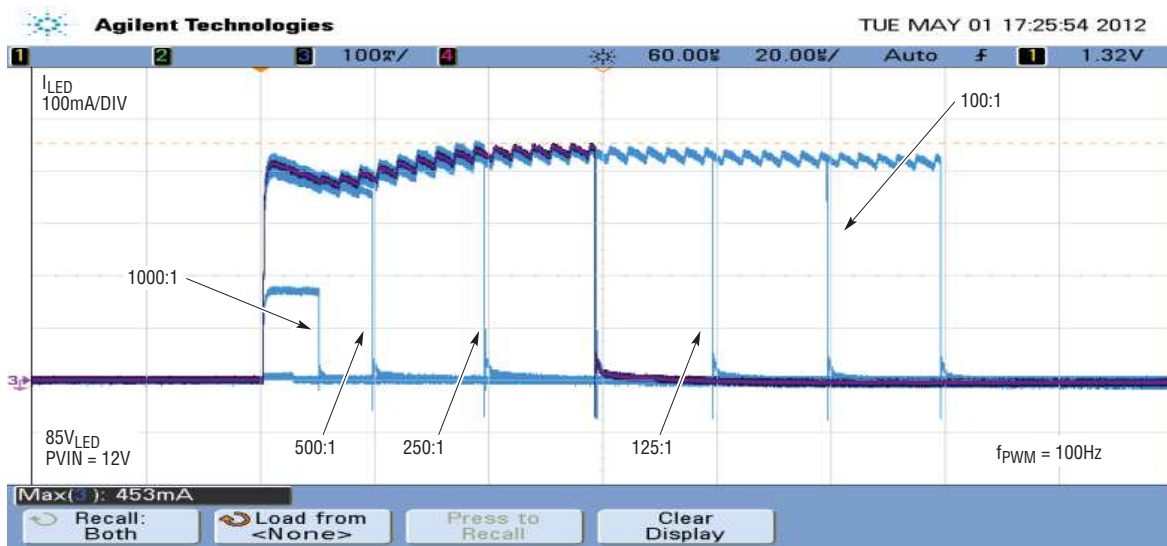
Figure 3. DC1706A 100Hz 100:1 to 1000:1 PWM Dimming Waveforms at 12V PVIN and 85V V LED
