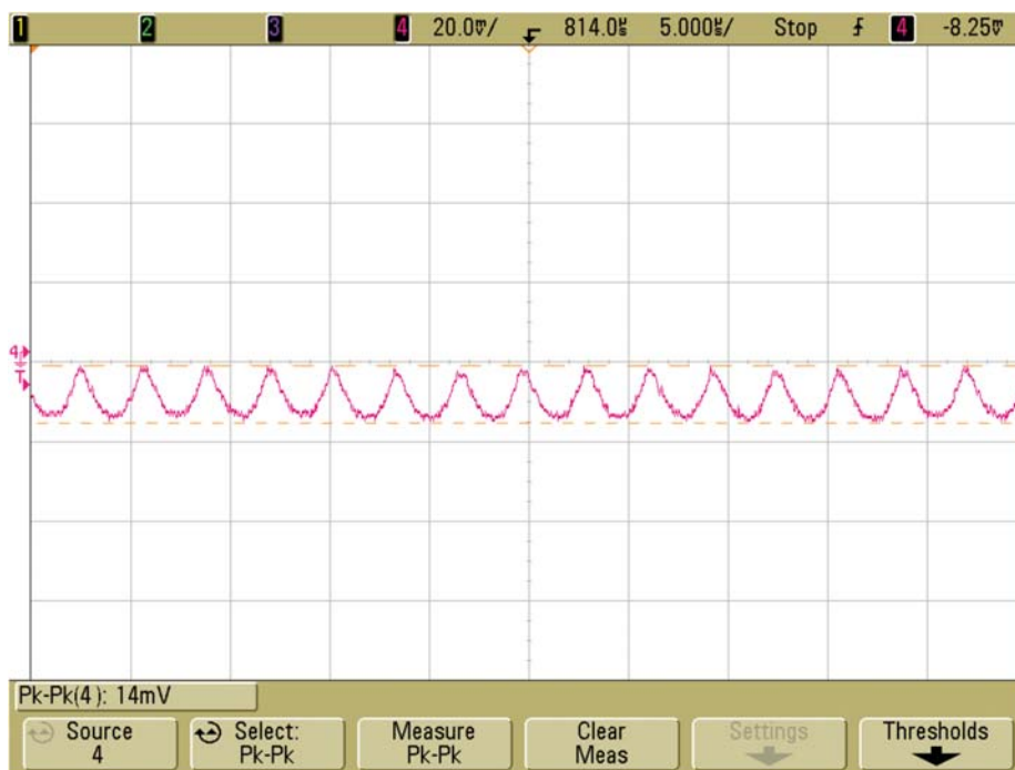
Figure 5. Output Noise, V_{IN} 4.5V , I_O 1A
