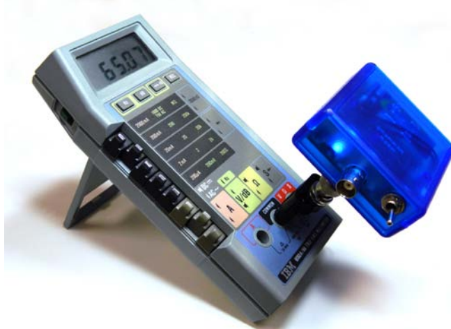
Figure 5. Completed Unit Attached to DMM
