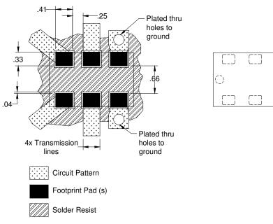
Dimensions are in Millimeters Mounting Footprint
