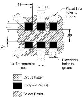
Dimensions are in Millimeters Mounting Footprint
