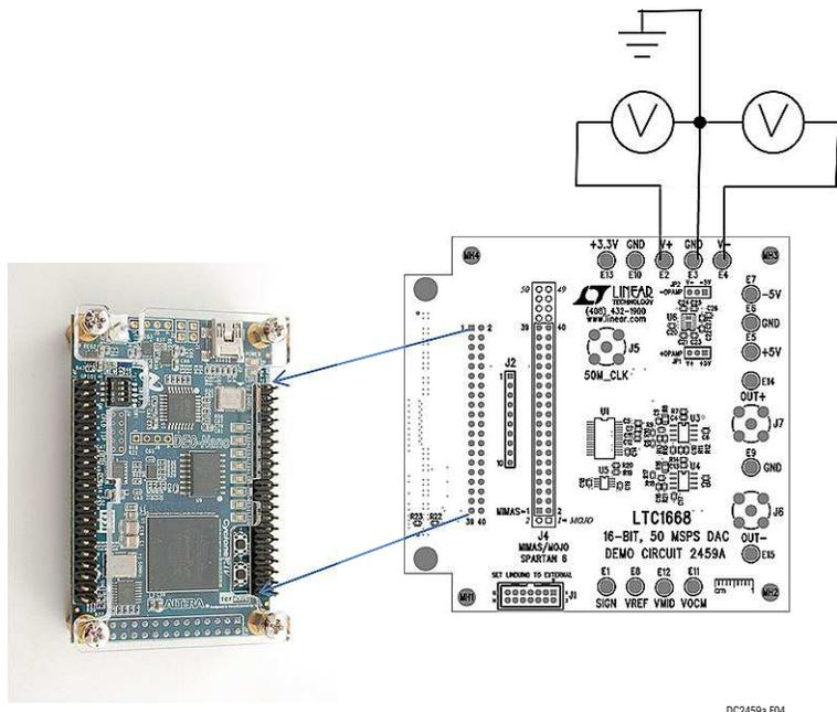
Figure 4. DC2459A Connected to the DEO Nano
