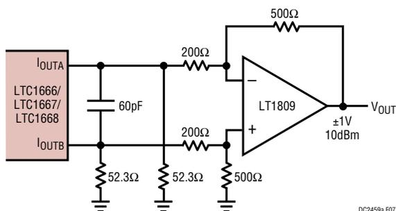
Figure 7. Differential to Single-Ended Op Amp I-V Converter
