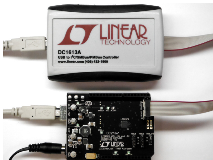
Figure 7. DC2467 with DC1613 Dongle Attached
