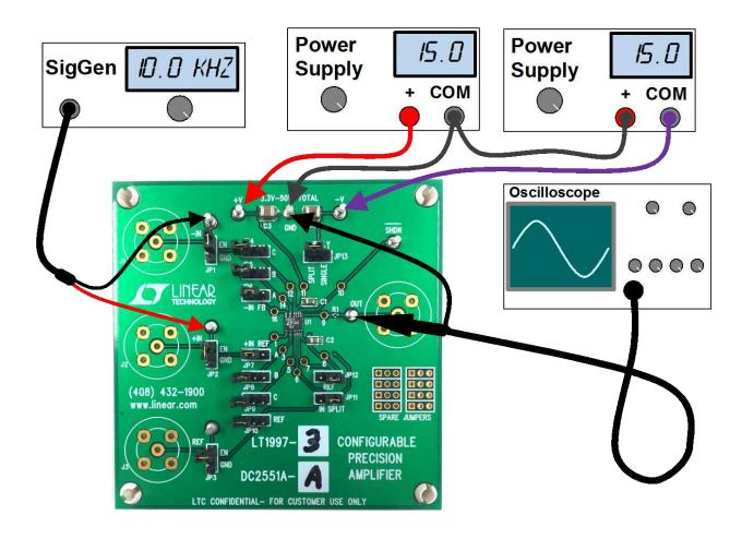
Figure 1. Proper Evaluation Equipment Setup
