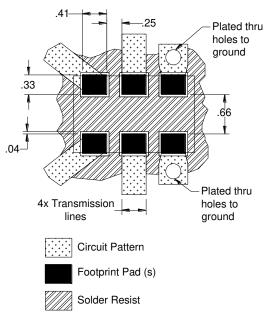
Dimensions are in Millimeters Mounting Footprint
