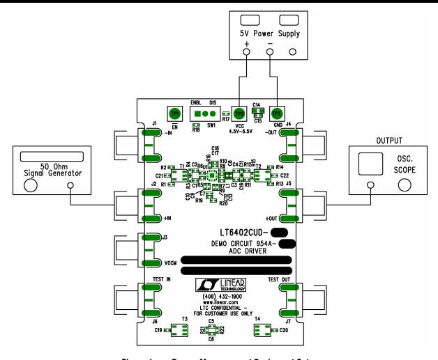
Figure 1. Proper Measurement Equipment Setup
