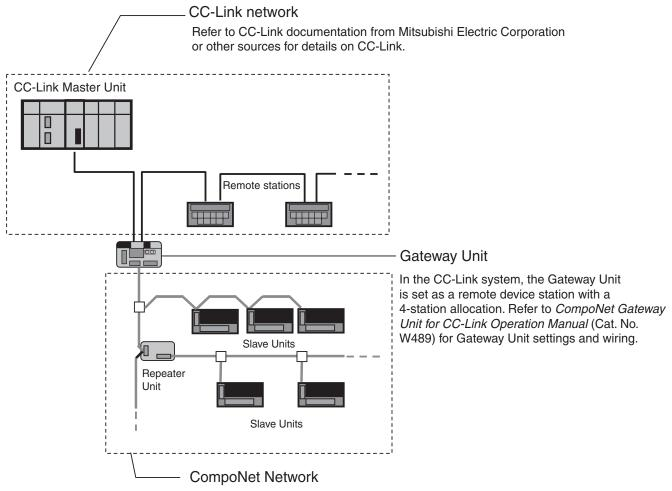
Refer to the *CompoNet Slave Unit and Repeater Unit Operation Manual* (Cat. No. W457) for the specifications of CompoNet networks. Refer to documentation for individual Slave Units and Repeater Units fordetails on those Units.
