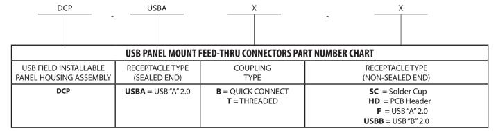
DCP-USBAB-\* mates with DCC-USBAB-150 or DCC-USBAB-180 DCP-USBAT-\* mates with DCC-USBAT-150 or DCC-USBAT-180
