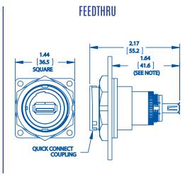
Note: Dimension does not include gasket compression. Dimensions in inches [mm]. Quick connect option shown. See drawings from Conxall.com for detailed dimensions
