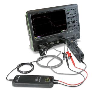
*CP150 150A current probe and HVD3106 high voltage differential probe connected to an HD06104A-MS 12-bit resolution high definition oscilloscope. The DCS025 is connected to the EXT input (to conserve analog channels) and the deskew amount is adjusted for one of the probes in the channel dialog menu. In this case, a vertical Zoom of the current signal is used for deskewing.*
