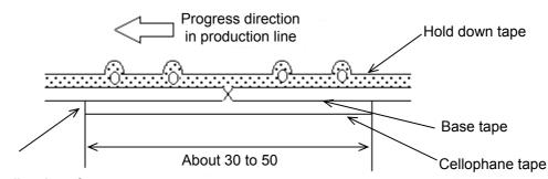
No lifting for the direction of progressing
