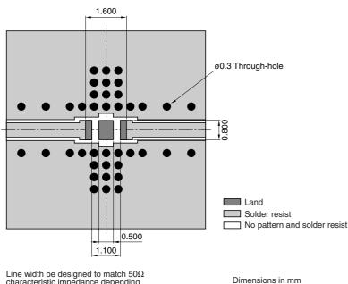
characteristic impedance depending on PCB material and thickness.
