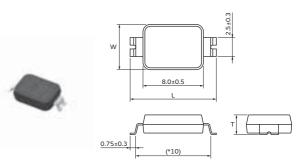
(in mm) L: 11.4±0.5, W: 6.0±0.5, T: 2.5 max. The value marked with \* is a reference.
