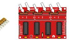
Solder one part at a time. Insert a part into the board, flip the board over, and solder one of the pins. Check to see if the part is still straight. If it isn't, re-melt the joint, and simultaneously straighten up the part. Once it's straight, solder the rest of the pins. You don't have to clip these pins unless you want to.
