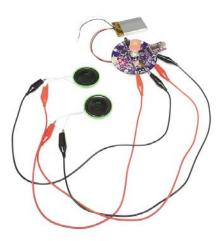
The LilyPad MP3 Player comes with preinstalled software called "**Trigger**" that will play specific files when the input pins are grounded. You can also add an optional rotary encoder and load the "**Player**" software to turn the board into a "real" audio player, or even write your own software using the free Arduino programming environment.
