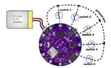
When you activate a switch, the trigger will be connected to ground, which is "low" or 0V. The software knows that when a trigger is low, it's time to play the proper audio file.
