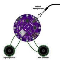
4. Connect a headphone to the headphone jack, **or** connect speakers to the left and right speaker terminals. (Note that when anything is plugged into the headphone jack, the speakers are disabled. This behavior can be changed if desired).
