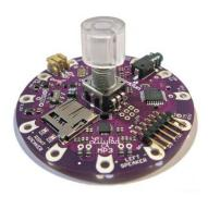
• Optional: place the knob onto the rotary encoder shaft. That's it!
