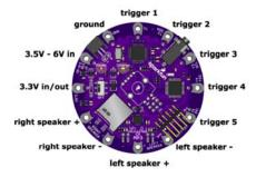
The LilyPad MP3 Player has **twelve "pins"** (they're really holes, but they connect to pins on the microcontroller) that you'll use to connect to the outside world. For each pin, we've provided both "**sew taps"** (large holes you can loop conductive thread around to use it in fabric projects), and standard **headers** (smaller holes that you can solder wires or header pins to if you wish).
