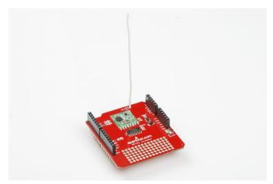
The RFM22 shield is an Arduino-compatible shield which provides a means to communicate with the HOPERF RFM22 radio transceiver module. What does THAT mean? It means you can use the RFM22 shield to add wireless communications to your Arduino projects.
