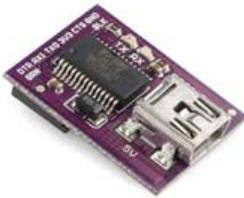
The FTDI Basic Breakout board is used to program the LilyPad Arduino Simple. This board can also be used to power the Development Board, or to charge a LiPo battery connected to the Arduino's white JST connector.
