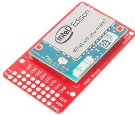
PWM Block Installed
