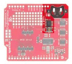
The Real-Time Clock is used to keep accurate time, which is often useful in security protocols. The clock on the CryptoShield is the DS3231M. It's attached to the I2C bus with an address of 0x68.
