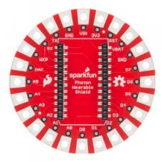
There are normal sized pins for soldering hook-up wire to the shield. Which, is great for projects needing tons of LEDs or a solid connection.
