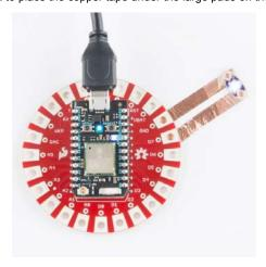
Use the copper tape with the large pins on the shield.
