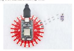
Tip: Loop around a large pin hole and component three or more times, with conductive thread, to get a solid connection.
