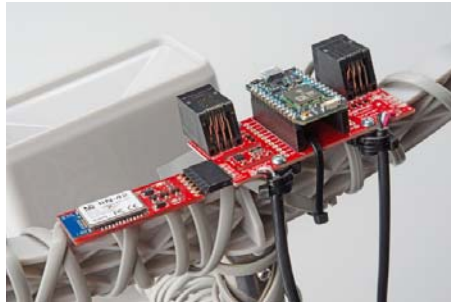
A BlueSMiRF connected to the Serial 1 Port using a 6-pin, right angle female header with the outermost pins removed.
