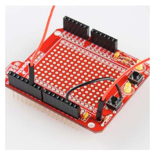
The **button** on the ProtoShield is '**pulled high**', meaning one side of the button is connected, through a resistor, to +5V and also to 'JC1' (which should then be connected to an Arduino pin of your choice). The other end of the button is simply connected to ground. This means that when the **button is pressed** it will **read as LOW**, otherwise it will be HIGH. In the example above, the LED will be on unless the button is being pressed.
