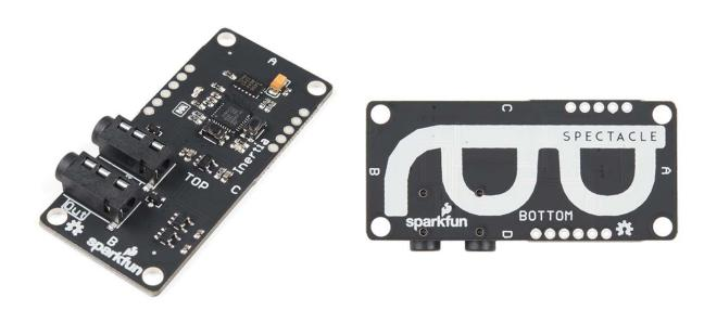
**Description:** The Spectacle Inertia Board makes it easy to sense motion or orientation with a Spectacle project. The Spectacle Inertia Board is designed to allow your Spectacle to detect whether it is moving or stationary, or whether it is under acceleration. At the heart of each Inertia Board is the trustworthy ADXL345 triple-axis MEMS accelerometer. The ADXL345 is a perfect fit for your Spectacle project when it comes to all things Inertia!
