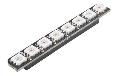
**Description:** The Pimoroni Blinkt! is a "shield" for the Raspberry Pi, equipped with eight superbright and addressable RGB LEDs that make it ideal for adding visual notifications to your Pi. Each LED is individually controllable and dimmable, allowing you to create gradients, pulsing effects, or just flash them on and off like crazy.
