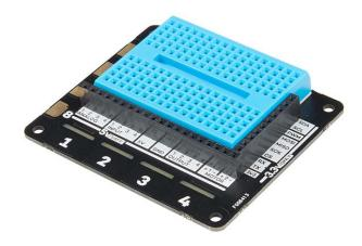
**Description:** The Pimoroni Explorer HAT Pro is a "shield" for the Raspberry Pi and provides you with the perfect prototyping sidekick for your Pi. The Explorer HAT Pro has a heap of useful input and output options that will take your Raspberry Pi projects to the next level. This add-on board is great for driving motors, using analog sensors, interfacing with 5V systems and touch (even fruit-based!) interfaces.
