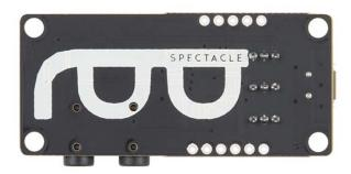
**Description:** The Spectacle Light Board allows you to add some fairly complex lighting effects to your Spectacle projects in a streamlined manner. Each has connections for you to add addressable LEDs as well as an external power connector. Designed to make it easy to add relatively complex lighting effects to your Spectacle projects, the Spectacle Light Board integrates with the rest of the Spectacle ecosystem to allow you to control lighting effects with ease and comfort.
