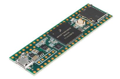
**Description:** The Teensy is a breadboard-friendly development board with loads of features in a, well, teensy package. Each Teensy 3.6 comes pre-flashed with a bootloader so you can program it using the onboard USB connection; no external programmer needed! You can program for the Teensy in your favorite program editor using C *or* you can install the Teensyduino add-on for the Arduino IDE and write Arduino sketches for it!
