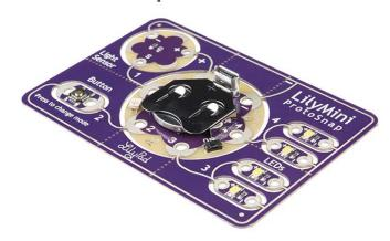
**Description:** The LilyMini ProtoSnap is a great way to get started learning about creating interactive e-textile circuits before you start sewing. Like other LilyPad ProtoSnap boards, the LilyMini ProtoSnap has all of its pieces wired together out of the box, enabling you to test the circuit's function before you sew. At the center of the board is a pre-programmed LilyMini microcontroller connected to a LilyPad Light Sensor, LilyPad Button and two pairs of LilyPad LEDs.
