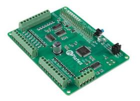
**Description:** The DAQCplate (Data Acquisition and Controller) from Pi-Plates adds a rich set of input/output options to your Raspberry Pi. It includes seven powerful digital outputs for driving external devices such as relays and high-current LEDs, as well as eight analog-to-digital inputs for measuring temperature, voltage, humidity and more. Additionally, there are eight digital inputs, two analog outputs and seven general-purpose indicator LEDs.
